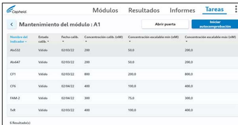
The screenshot shows the 'Mantenimiento del módulo' screen for module A1. It features a table with the following data:
