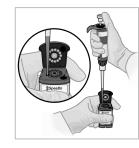
8 Gently tap bottom of cartridge on bench to settle liauid and prevent any air bubbles.
