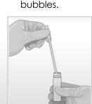
10 Transfer pipette into the Sample Chamber (right), and slowly compress bulb to release sample
