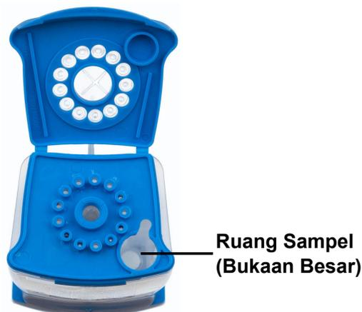
**Gambar 3. Xpert HIV-1 Qual XCKartrid (Tampak Atas)**
