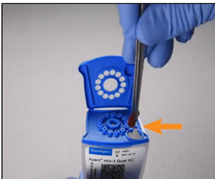
Figure 5. Insertion of DBS into Sample Chamber
