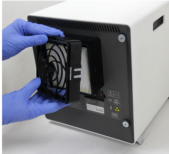
Gambar 9-27. Melepaskan Penahan Filter HE
