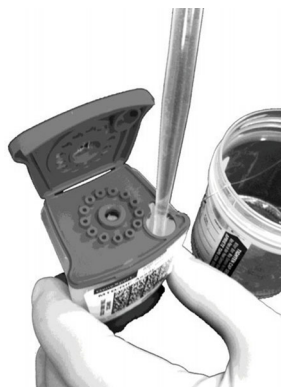
Figure 5. Dispensing Decontaminated Liquefied Sample into the Sample Chamber of the Cartridge
