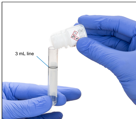
Figure 4. Example of 2:1 Dilution (2 mL SR:1 mL Sputum)
