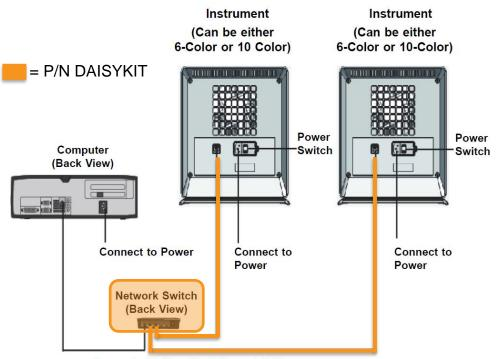
Connect with Supplied Ethernet Cables
